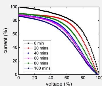
IV curves and cell parameters of an unencapsulated PSK cell are measured after various degradation times at 65 °C in air and 35% humidity.
